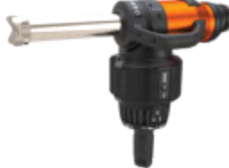
Single Plunger Ram PRA40 1st plunger: 30574 lbf max Weight: 31.3 lbs. Retracted : 15.2 / Extended: 23.6
