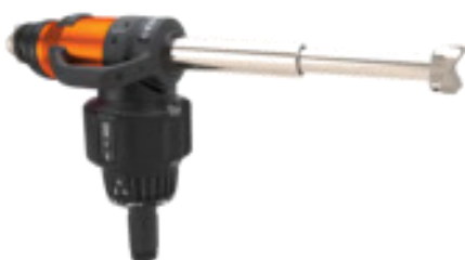
Telescopic RAM PTR40 1st plunger: 30574 lbf max 2nd plunger: 14613 lbf max Weight: 34.2 lbs. Retracted : 15.92" / Extended: 31.2
